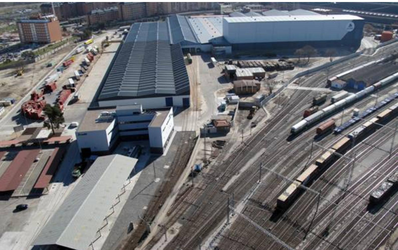
For the construction of the North-Northwest High Speed corridor superstructure on the Ourense - Santiago stretch, it was necessary to build a track assembly base and ballast stockpiles, which would also serve as a maintenance base for both UIC gauge and conventional gauge machinery.
